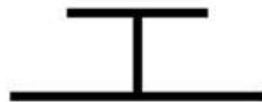
'H' trim - provides a low profile joint within a floor. It provides for expansion as well as locating the flooring.
