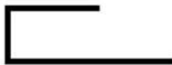
End trim - used to adjoining floor surfaces at the same height or along sliding patio door tracks.
