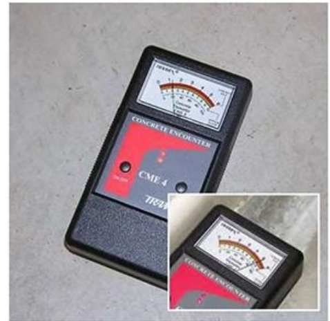
Concrete impedance moisture meter. The inset shows the meter detecting slab edge dampness.
