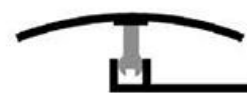
'T' trim - used to provide a smooth transition to two different floor surfaces that are at different heights.
